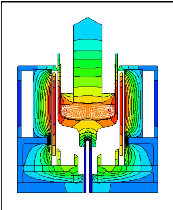
The simulator for the Liquid Encapsulated Czochralski (LEC) system has been developed to model industrial scale growth of GaAs and InP. It is based on pioneering work done at MIT, and can be adapted to geometric details of all commercial and custom furnaces. The simulation results have been extensively validated by experimental measurements.
